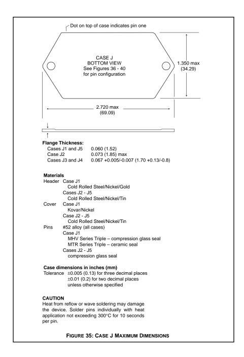
Note: Although every effort has been made to render the case drawings at actual size, variations in the printing process may cause some distortion. Please refer to the numerical dimensions for accuracy.
